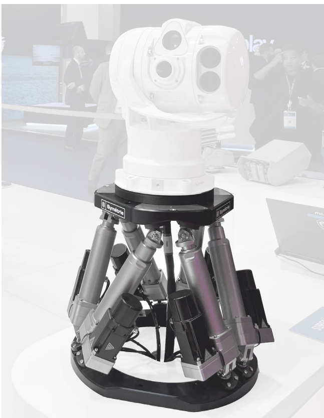
HEGOA hexapod testing the motion compensation performances of a gyro stabilized platform.
